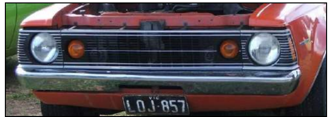
Grille with silver centre line, the same as above left, but orange indicators not clear ones
